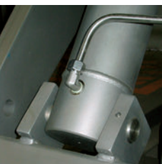
Cylinder with built-in safety valve.
