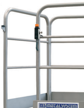
Safety handrails with kick plates and access gates with safety mechanism (lift table will not work if gate is open).
