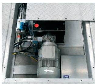
Maintenance hatch providing access to the hydraulic motor when the lift table is in its folded position.
