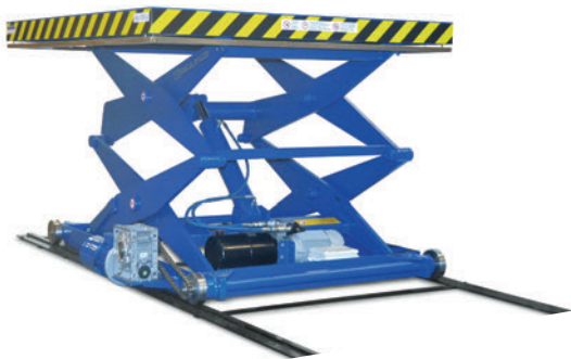
Double-scissor lift table with sideways movement on rails. Motor with encoder for precision positioning.
